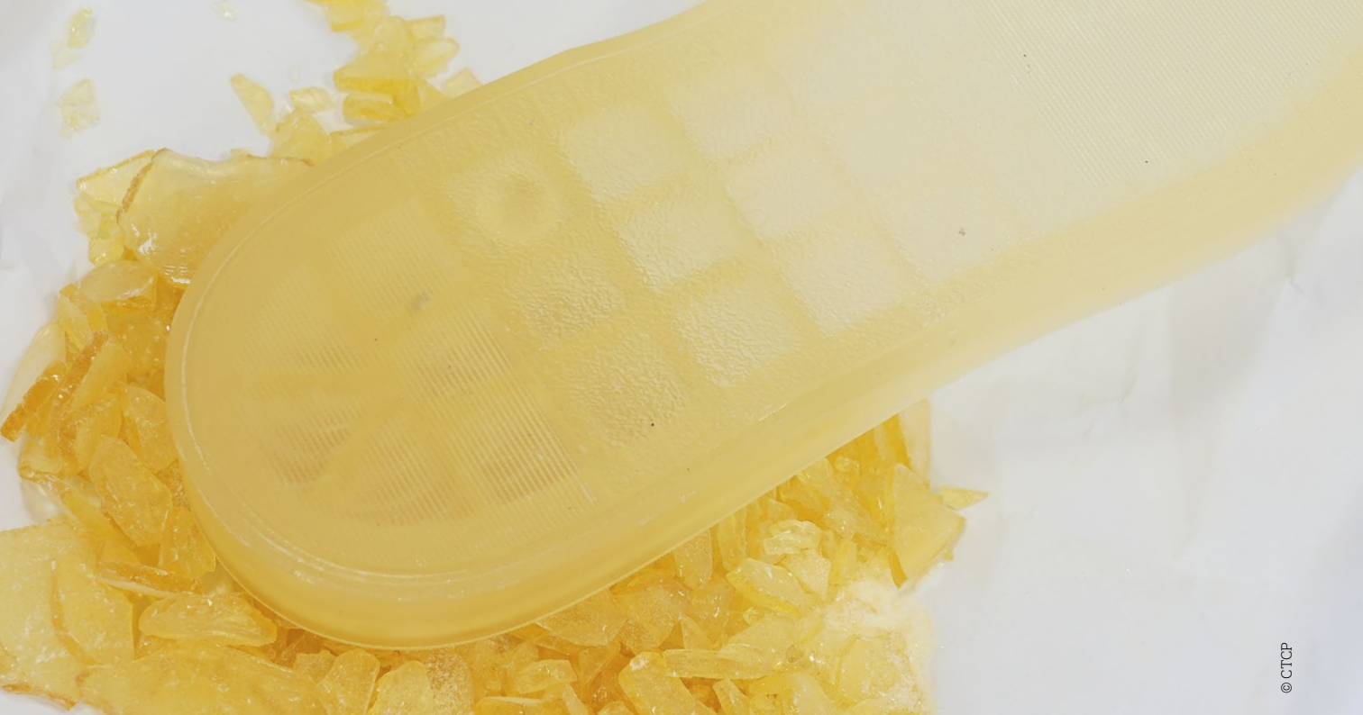
Figure 4 - Sole with 15% resin in its composition.
