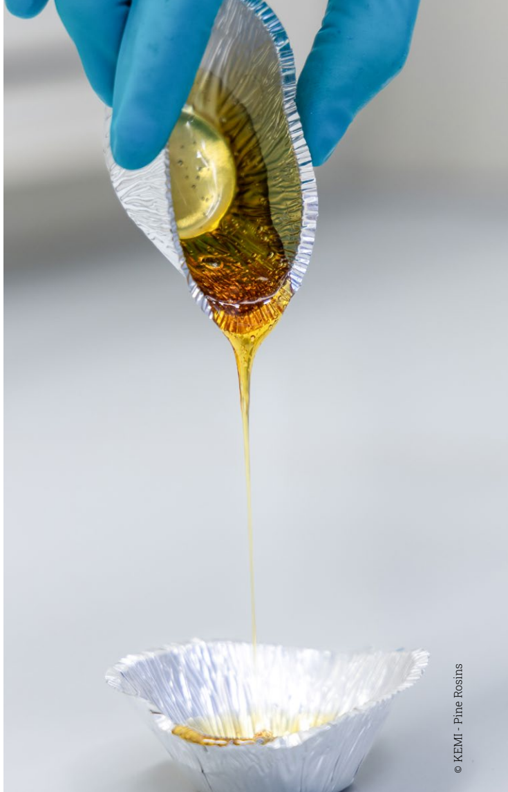
Figure 4 - Semi-solid polyamide at room temperature, with a softening pint of 67°C without tackifier.
